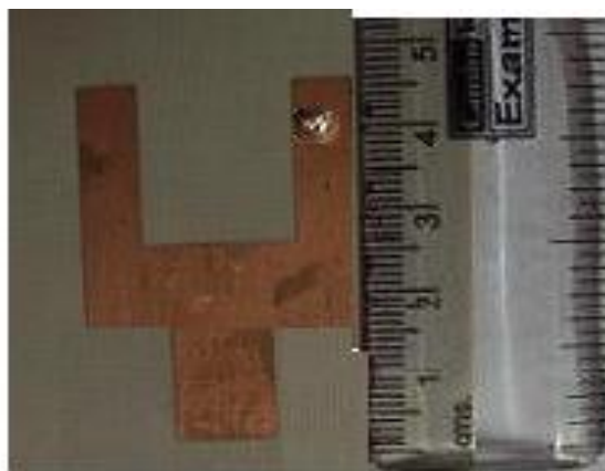
Figure 4. Front view of fabricated proposed Fork slot antenna
